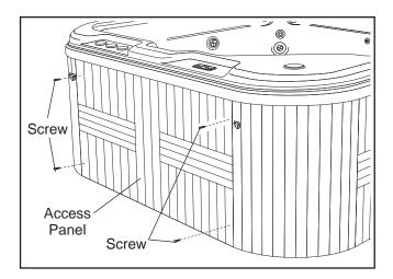
To re-attach the access panel, insert the top of the access panel under the edge of the spa shell. Slide the access panel up until the bottom of the access panel clears the trim along the bottom of the spa. Then, slide the access panel into place and re-attach it with the four screws.
